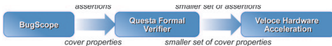
Figure 3 Assertion Synthesis Driven Hardware Acceleration Flow
